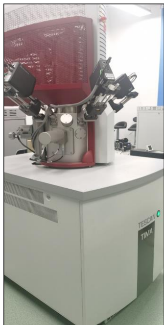
SEM TESCAN MIRA3 LMH/ TIMA X 配备探头 TESCAN BSE探头 TESCAN CL探头 EDAX Element 30*4
